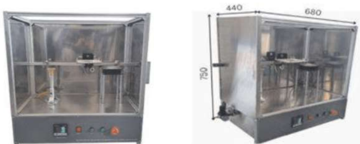
Fig. 9.3: Specification & design of fabrication of convective heat tester
