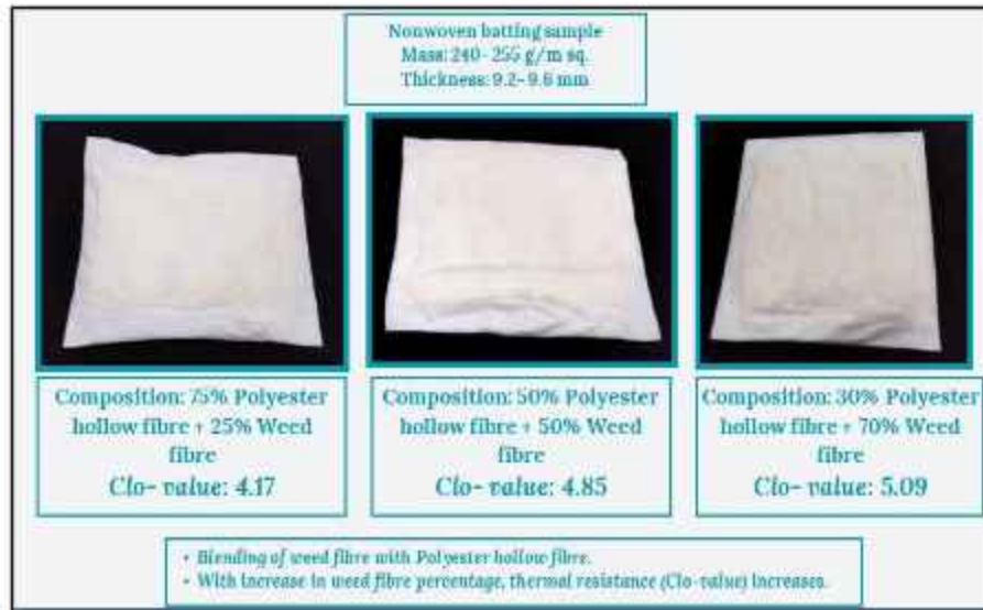
Fig. 22 (b): Blended nonwoven samples developed at NITRA Nonwoven Pilot Plant
