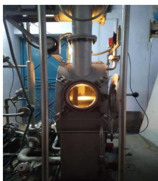
Fig.1: Soft flow dyeing machine used for cotton hank dyeing
