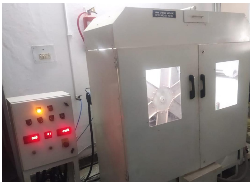
Fig.5 : Pilot model of newly developed Hank Dyeing Machine
