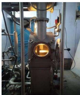
Fig.5: Soft flow dyeing machine used for
