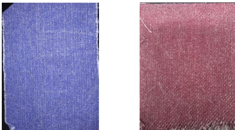
Fig.4 : Cotton Fabrics having denim effect created by using disperse dye
