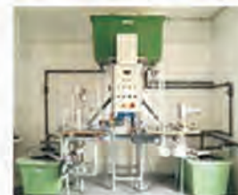
Water Permeability: In the plane of the geosynthetic (with load)
