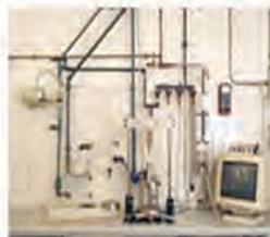
Water Permeability: Perpendicular to the plane of the geosynthetic (with load)
